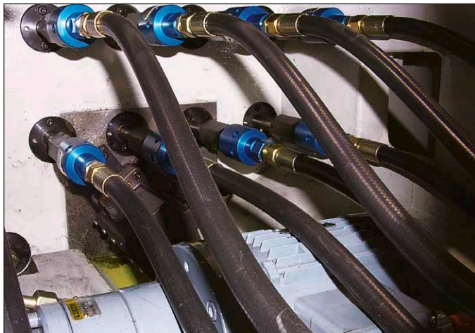
Deublin 1116 Bearing-Supported Unions on Automotive Transfer Line.
